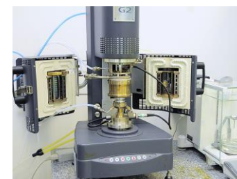
rheometer AR-G2 (TA Instruments) T Ambient at 600 °C
