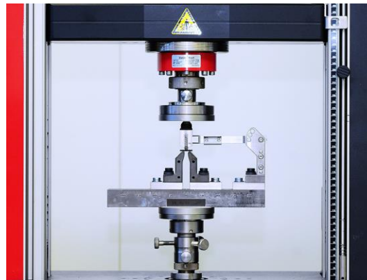
Universal Testing Machine: Zwick AllroundLine Z010TH Room temperature Range: 10kN
