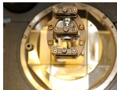
Dynamic mechanical analysis, DMA Mod. Q800 DMA (TA Instruments-Watters LCC) Range: -145°C to 600°C
