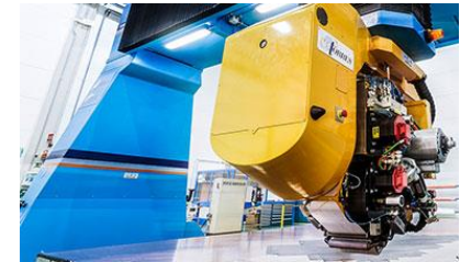
Automatic tape laying(ATL) with ultrasonic panex cutter included
