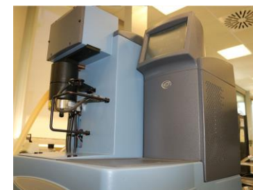
Thermogravimetric analysis, TGA Mod. Q500 TGA (TA Instruments-Watters LCC) Range: T Ambient to 1000 °C
