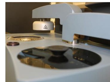
Differential Scanning Calorimeter, DSC Mod. Q2000 DSC (TA Instruments-Watters LCC) Range: -90°C to 55°C
