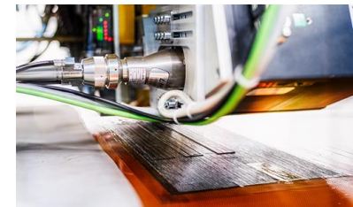
IN SITU consolidation thermoplastic AFP
