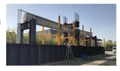
The Center also has exclusive equipment in Italy for testing **real-size structural elements** with lengths of up to 30 meters, which can be performed using **a modular and transportable steel reaction frame** (equipped with a load application systems with 4 actuators of 1200 kN each).
